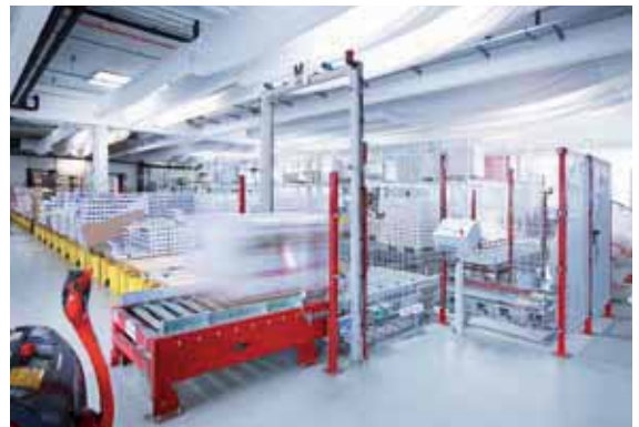
Control station to check loads and load carriers for profile, overloading and overhang.
